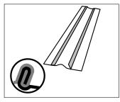
3. Using heavy snips, notch standing seam at bend points.
