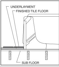
Below is shown typical cross sections of the tub rim showing typical wall constructions.
