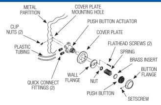
Using Cover Plate as a template, drill two 3/16" (5 mm) Cover Plate Mounting holes and cut opening for Push Button Actuator into the metal partition. Install Clip Nuts with threaded side toward
