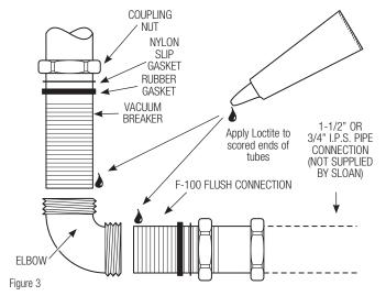
Loctite can also be used to secure Push Button Flange. See Sealant package for details.
