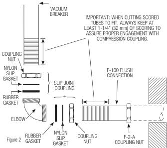
**IMPORTANT:** Before inserting the scored ends into the Elbow, apply several drops of Loctite (supplied by Sloan) to the scored ends of the tubes (Figure 3). This sealant helps prevent separation under high-pressure conditions. **DO NOT** use any other pipe sealant or lubricant on this connection.
