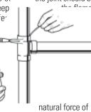
capillary attraction. When the joint i s filled, a continuous fillet of brazing alloy will be visible completely around the joint. Stop feeding as soon as the joint is filled, using table on page 54 as a guide for the alloy consumption.
