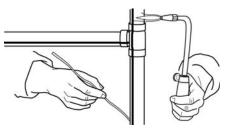
hard against the stop. The assembly should be firmly supported so that it will remain in alignment during the brazing operation.
