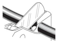
Insert fitting into tubing, then position crimp ring squarely over barbs. Proper alignment is important for making the best connection.
