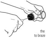
a contaminated or an improperly cleaned surface will result in an unsatisfactory joint. Brazing alloys will not flow over or bond to oxides; and oily or greasy surfaces tend to repel fluxes, leaving bare spots which will oxidize, resulting in voids and inclusions.
