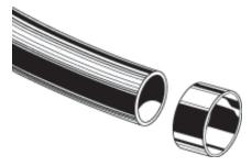
4. Center the crimping tool jaws exactly over the ring, and bring the tool handles together until totally closed to the stop indicator. Check each crimp ring with the caliper gauge after completion. If the small flats on the gauge do not fit over the crimped ring, the ring is undercrimped. Cut out any undercrimped rings and fittings, and completely replace.
