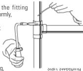
When the flux appears liquid 9. on both the tube and the fitting, the flame back and forth along the axis of the joint to maintain heat on the parts to be joined, especially toward the base of the cup of the fitting. The flame must be kept moving to avoid burning the tube or the fitting.
