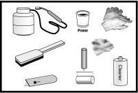
Propane tank, hose, torch & regulator. Appropriate tools for surface abrasion. Knife, roller, rags & approved cleaner. Wire brush, paint brush or paint roller, tape measure, and marker. Standard safety equipment; gloves, goggles, hard hat, etc.
