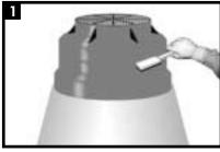
Ensure all surfaces which the sleeve will be applied to are clean, dry and free of foreign objects and sharp edges.
