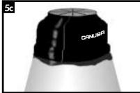
At the overlap, ensure that the top and bottom edges of the sleeve are uniformly aligned.
