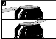
After shrinking, WrapidSeal <sup>™</sup> will be draped over the manhole frame gussets. Using a knife, cut the sleeve around the gussets. Apply gentle heat and press the sleeve onto the steel frame. Trim excess material protruding above the steel manhole frame and cover.
