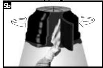
Remove ~6" of the release liner from the sleeve. Using the perimeter marks as a guide, begin wrapping the sleeve around the manhole while gradually removing the release liner.
