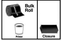
WrapidSeal is typically shipped in bulk rolls. Closures are shipped pre-cut. The adhesive is protected from contamination by an inner liner. Primer is sold separately.
