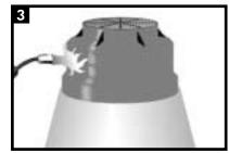
Using the torch, warm the surface to drive off any moisture.
