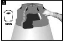
Apply WrapidSeal<sup>™</sup> Primer to the application surfaces, (i.e. steel, concrete, fiberglass etc.) Wait until the primer is slightly tacky to touch before proceeding. This will take 5-15 minutes depending on temperature and humidity conditions.
