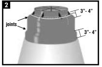
WrapidSeal<sup>™</sup> should be sized to extend 3" - 4" above and below the upper and lower joints of the cone section, grade rings and frame. As a guide, make a series of marks around the manhole where the bottom of the sleeve will be. Determine the layflat length of the sleeve by measuring the circumference of the manhole structure at the marks and add the overlap dimension, (6" minumum).
