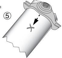
Step 6 • Install U-bolt(s) on saddle body, and tighten finger tight. Make sure the gasket has seated itself flat on the pipe face.
