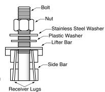
Step 6 • Well-tightened nuts are important to ensure a full-circle seal. Tighten nuts, starting with center bolts, alternating on either side of the sleeve. Gap between sleeve halves on either side should be the same when nuts are fully torqued.
