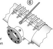
Tighten nuts evenly in 25 ft-lb. increments. After reaching the appropriate torque on the final nut, retighten all nuts using the same alternating pattern, to the minimum torque value listed below.
