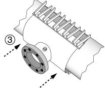
Step 4 • Bring back half of sleeve into position, making sure bolts are located between mating receiver lugs on the sleeve outlet half. Check gasket edges along sleeve top and bottom halves to be sure they overlap and are not folded under. Also check that the armor is between the back half and pipe.
