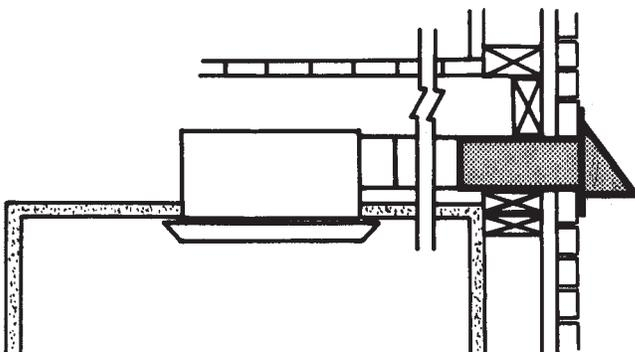
BRICK CONSTRUCTION: Position cap so that it will be flush with outer surface of brick. Nail in place through throat of cap. Connect fan to cap with 3" round duct. Tape all duct connections. Caulk around flange.
