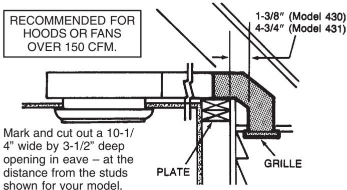
Mark and cut out a 10-1/4" wide by 3-1/2" deep opening in eave – at the distance from the studs shown for your model.
