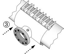
Step 4 • Bring back half of sleeve into position, making sure bolts are located between mating receiver lugs on the sleeve outlet half. Check gasket edges along sleeve top and bottom halves to be sure they overlap and are not folded under. Also check that the armor is between the back half and pipe.
