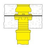
With Flange -F and Flashing Fig. 8 Clamp -C
