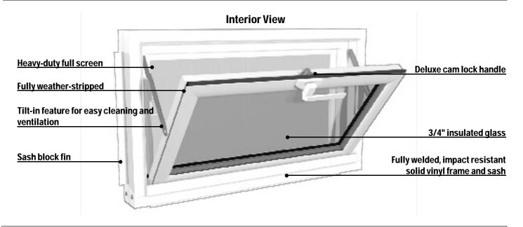
IMPORTANT – PLEASE READ Duo-Corp.'s Vinyl Basement Window is a Hopper-Type window that opens to the inside. It is ABSOLUTELY ESSENTIAL that the window be installed with the locking handle to the inside and at the top of the window.
