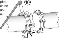
**NOTE:** Do not turn a bolt more than one turn before alternating to the next bolt.
