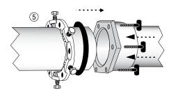
**Step 6** • Tighten T-bolts to the torque recommended in AWWA C111. Maintain the same overall gap between the RG-PVC and the MJ bell face by tightening the T-bolts in a uniform criss-cross pattern (12 o'clock, 6 o'clock, 3 o'clock, 9 o'clock) until proper torque is achieved. Using a torque
