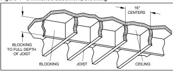
Figure 5- Unfinished Basement, Branch Line Support
