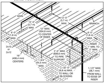
Figure 2 – Unfinished Basement, Center Wall Riser with Main at Wall
