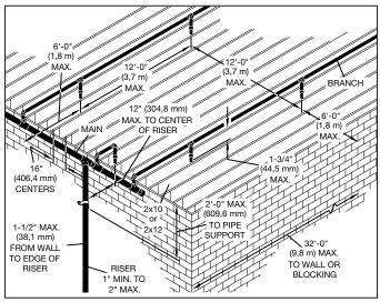
Figure 3 - Unfinished Basement, Riser in Corner
