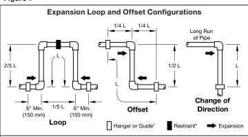
\* Hangers should only be placed in the loop, offset, or change of direction as indicated. Piping supports should restrict lateral movement and shall direct axial movement into the expansion loop.
