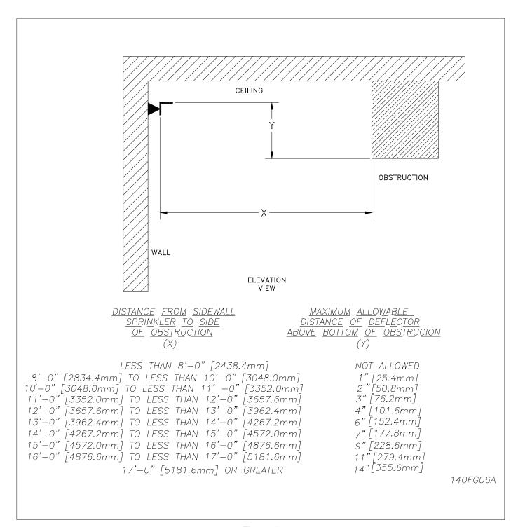
**Figure 6**Positioning of sidewall sprinklers to avoid obstructions.
