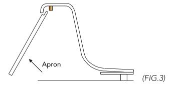
4. Insert the lip of trimmed apron up under tub edge, between the wooden blocks and the front tub lip. Check to see that you have cut the apron to the proper height. Remove apron.
