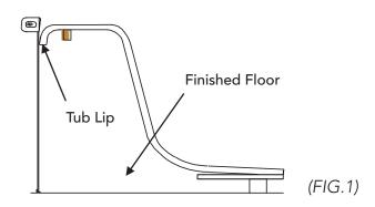
1. With soaking tub or whirlpool in place, measure from the bottom of the tub lip to the finished floor surface. Subtract 1/8" from this dimension for clearance. This adjusted dimension will be used to determine the proper apron height for your installation.
