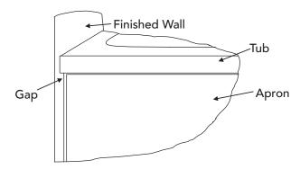
Note: Final installation will leave clearance between both ends of apron and finished wall to allow for future removal.
