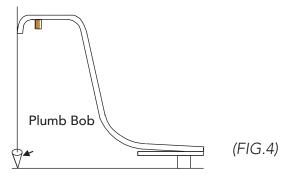
5. Using a plumb bob or level, project front edge of tub lip down to floor surface and make a mark on floor. Repeat several times across front of tub. Draw a straight line at these marks.
