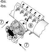
**Step 8** • Remove test plug and connect test apparatus to tapping sleeve assembly. Test at pressure up to 1.25 times the pressure in the pipeline or to the maximum in the table (below), whichever is less. If assembly leaks, check bolts to be sure the nuts have been torqued to the recommended torque value and then retest assembly.
