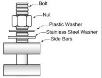
**Note:** On 4" nominal SSTIII's install sleeve bolts with the bolt heads facing the flange for more flange bolt clearance.
