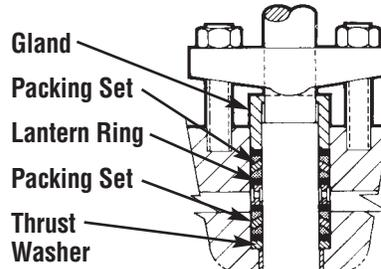
**Adjuster Fastener Torque — Fire Sealed Grafoil Packing**
