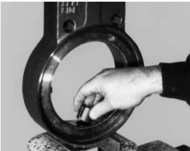
2. Place one disc thrust washer over the bearing and then place the disc (disc pin slot up toward the top end of the valve body) into the valve body, aligning the disc and body shaft bores. Slide the second disc thrust washer into the gap between the top of the disc and valve body.
