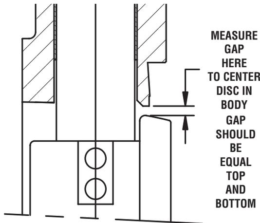
13. For valves with an external disc support design, assemble the disc support hardware on the bottom of the valve body. See **Figure 4**.
