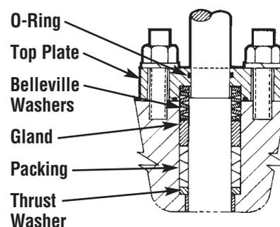
**Adjuster Fastener Torque — PTFE Cup and Cone Packing**
