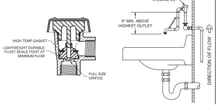
**CAUTION:** This device should never be used in installations that are under continuous pressure. Therefore, never place a shut-off or check valve downstream of AVB's. This device shall not be installed in a concealed or inaccessible location, nor where the venting water from the device during normal functioning may be deemed objectionable.
