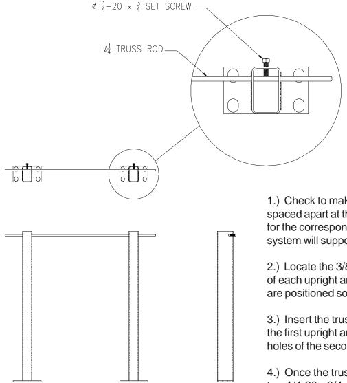
1.) Check to make sure that the uprights are spaced apart at the correct rough-in dimension for the corresponding fixture that the carrier system will support.
