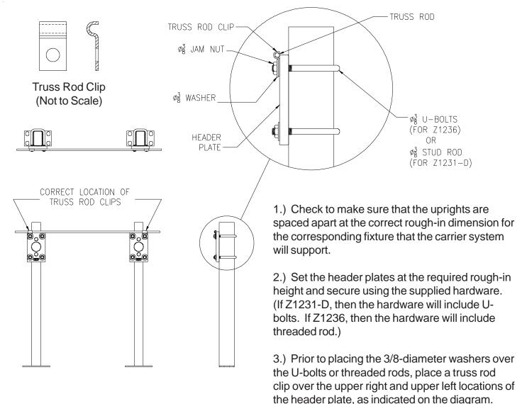
4.) Place a 3/8-diameter washer over the truss rod clip and proceed to place washers on all other remaining studs or U-bolts.
