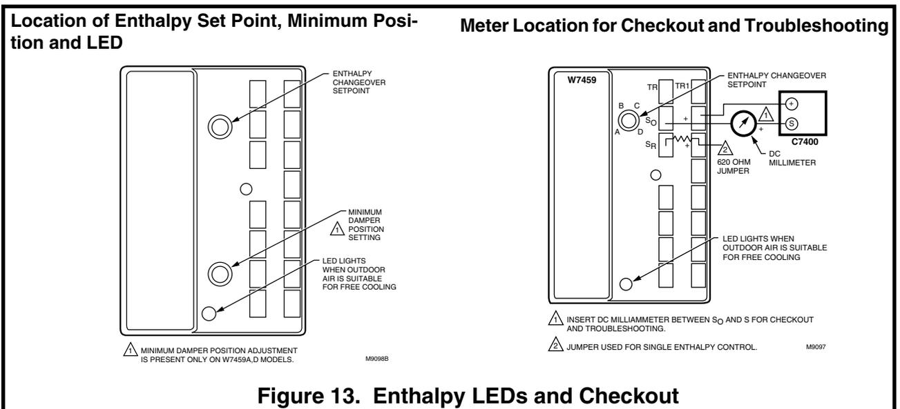
**Figure 13. Enthalpy LEDs and Checkout**
