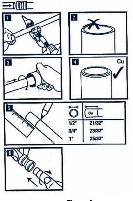
Figure A QTITE Copper and CPVC Installation
