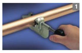
1) Cut the tube square. Use a rotary tube cutter whenever possible. If a hacksaw is used to cut the tube, then file the tube end exterior and interior using a fine tooth file. Care should be used to remove and smooth all burrs.
