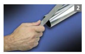
2) Remove burrs at the tube ends before insertion into a fitting. Internal and external tube ends should be deburred by use of a fine tooth file. The tube end should then be wiped clean of all debris to avoid damage to the o-ring upon tube insertion.
