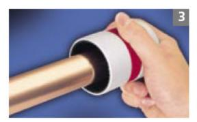
3) Commercially available deburring tools may be used to insure a smooth interior and exterior at the tube end. EPC markets deburring tools particularly well suited to performing this operation.
