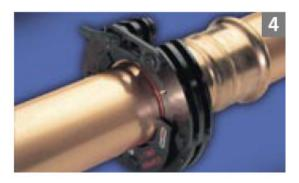
4) Turn the catch mechanism toward the locking pin. Depress the pin and push the catch into the pin until the mechanism engages. Revolve the pressing ring around the fitting to the desired position.
