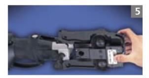
5) Attach the appropriate adapter to the press tool and close the breach bolt. Attach the adapter to the pressing ring by depressing the jaw levers and inserting the claws as far as possible into the grooves of the pressing ring. Do not press the joint until the adapter is correctly connected to the pressing ring.
