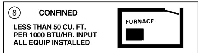
1. All air from inside the building as in Figure 9: The confined space shall be provided with two permanent openings communicating directly with an additional room(s) of sufficient volume so that the combined volume of all spaces meets the criteria for an unconfined space. The total input of all gas utilization equipment installed in the combined space shall be considered in making this determination. Refer to Table 3, for minimum open areas required.
