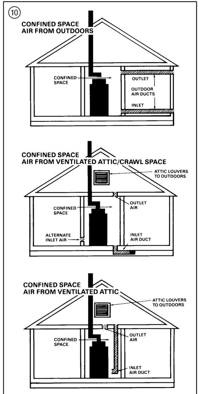
3. The following types of installations will **require** use of **OUTDOOR AIR** for combustion, due to chemical exposures:
