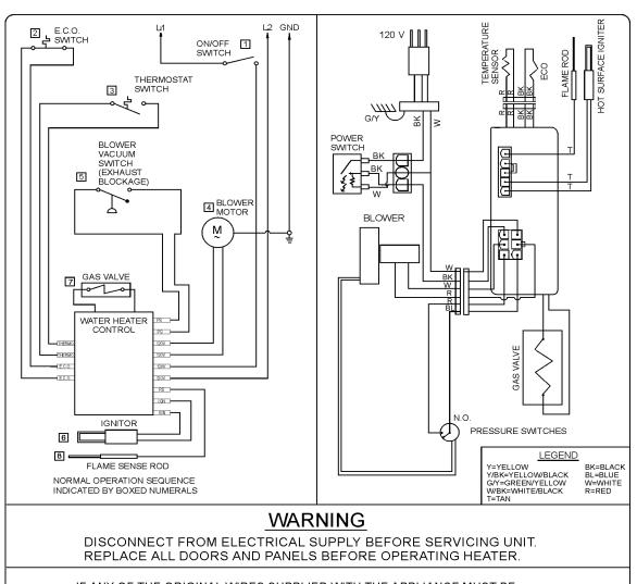
IF ANY OF THE ORIGINAL WIRES SUPPLIED WITH THE APPLIANCE MUST BE REPLACED, IT MUST BE REPLACED WITH APPLIANCE WIRE MATERIAL WITH MINIMUM TEMPERATURE RATING OF 105°C AND A MINIMUM SIZE OF NO. 18 AWG.
