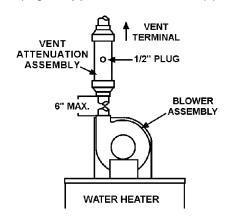
FIGURE 22: Typical Vertical Installation
