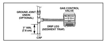
FIGURE 12. GAS PIPING WITH FLEXIBLE CONNECTOR.
