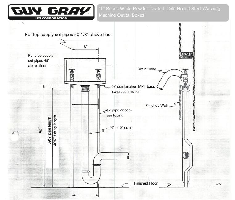
Plumbing rough-in measurements for space saver Washing machine supply and drain—Model T-150 & T-200
