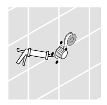
Install the anchors. Seal the wall around the anchors with waterproof sealant.
