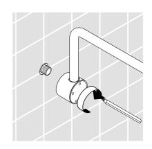
Wrap the threads on the nipple with Teflon thread tape. Seal the wall around the nipple with waterproof sealant.
