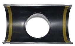
1. Bentonite placement - first two strips. Cut the first two strips of the bentonite sealing tape. Remove the protective paper. Apply the tape to the underside of the saddle keeping it centered under the band areas. SEE DETAIL.
