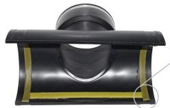
2. Bentonite placement - second two strips. Cut the second two strips of bentonite sealing tape. Remove the protective paper. Apply the tape to the underside of the saddle, 1/2" from each edge. Butt up to the first two strips. **DO NOT overlap.**
