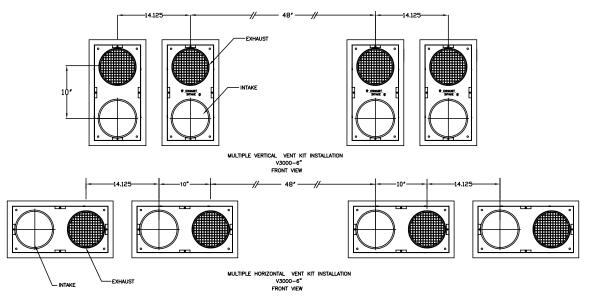
Fig. 5-3 Multiple Stainless Steel Horizontal Vent Kit Installation – Front View
