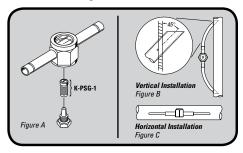
All Parker Sight Glass indicators are suitable for use with the halocarbon refrigerants, including 11, 12, 22, 113, 114, 134a, 404A, 407C, 410A, 502 and 507. Listed by Underwriter's Laboratories, Inc. for a working pressure of 650 psig or 4482 kPa.
