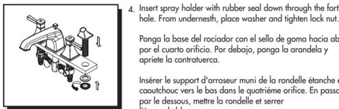
4. Insert spray holder with rubber seal down through the fourth hole. From underneath, place washer and tighten lock nut.
