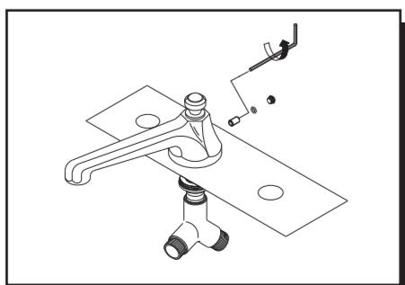
3. Install the spout and tighten the set screw in the back of the spout.
