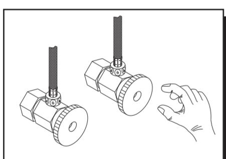
1. Turn off the water supply. Remove the old faucet making sure not to damage the water lines.
