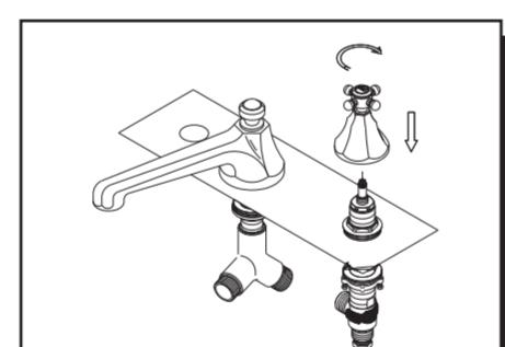
4. Place the handle body through right hole. Re-assemble the parts and screw with lock nut.
