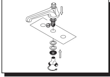
2. Apply plumber's putty around bottom of spout. Place spout in center hole of sink. Secure with pictured parts.
