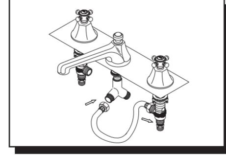
5. Connect handle body and faucet body with water supply tube and tighten with lock nut.
