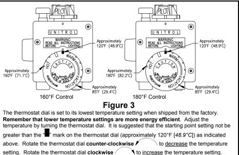
Adjust the dial until the minimum acceptable temperature is achieved (See figure 3 above for approximate temperature settings).
