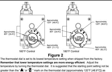
indicated above. Rotate the thermostat dial **clockwise** to <u>decrease</u> the temperature setting. Rotate the thermostat dial **counter-clockwise** to <u>increase</u> the temperature setting. Adjust the dial until the minimum acceptable temperature is achieved (See figure 2
