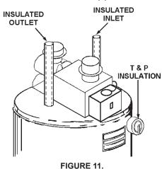
Fit pipe insulation over the incoming cold water line and the hot water line. Make sure that the insulation is against the top cover of the heater. Fit T & P valve insulation over valve. Make sure that the insulation does not interfere with the lever of the T & P valve.
