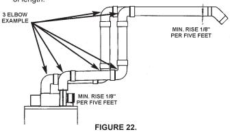
2. The total vertical and horizontal vent runs cannot exceed the maximum length with the number of 90° elbows as specified in the table below. If more elbows are required, the venting distance must be reduced 5 feet (1.5m) for every 90° elbow:
