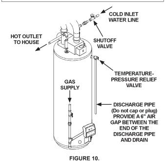
Figure 10 shows the typical attachment of the water piping to the water heater. The water heater is equipped with 3/4 inch NPT water connections.
