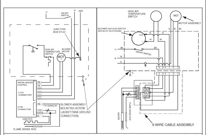
You must provide all wiring of the proper size outside of the water heater. You must obey local codes and electricity utility requirements when you install this wiring. This appliance is polarity sensitive. Outlets and field installed power supplies must have correct polarity or the water heater will not operate.
