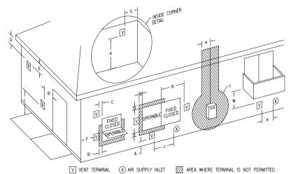
Figure 4 Direct Vent Terminal Clearances
