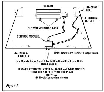
IMPORTANT: Ground lead must be connected to the green screw located on the junction box. Failure to do so will prevent the appliance from operating. The appliance must be electrically grounded in accordance with local codes or, in the absence of local codes, the National Electrical Code, ANSI/NFPA 70-(latest edition). (In Canada, the current CSA C22-1 Canadian Electrical Code.)
