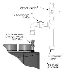
Figure 5.1: Gas Supply Pipe and Shut-off
