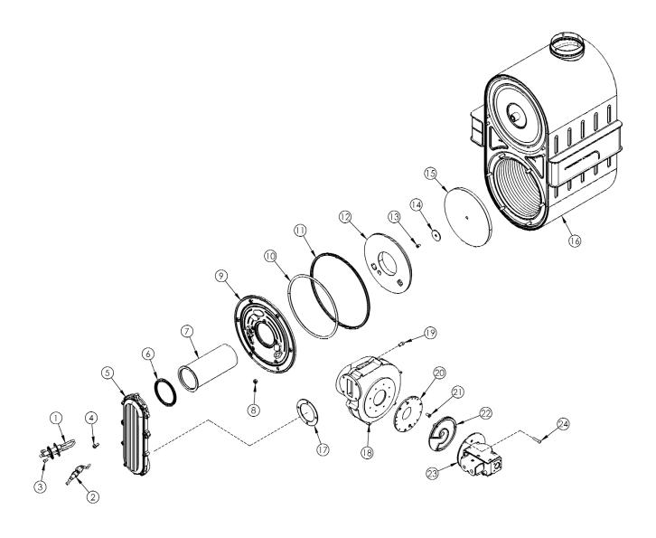
Figure 13.4: Heat Exchanger/Burner Assembly Repair Parts - PF-210 & PF-399
