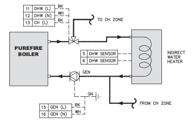
Figure 8.4: Pump Mode = 1, DHW Mode = 1 or 2
