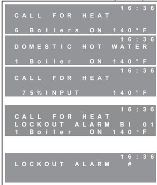
Call For Heat (Master Cascade Boiler): The Master boiler will display "CALL FOR HEAT" if there is a central heating demand and "DOMESTIC HOT WATER" for a DHW demand. The number of boilers currently running is shown at the bottom of the screen in addition to the current System temperature.
