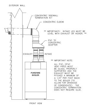
Figure 3.8: Optional Concentric PVC Vent Kit Installation
