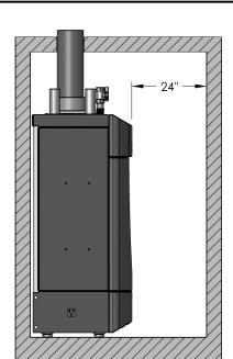
2. Figure 1.1 shows the minimum recommended clearances to allow reasonable access to the boiler for Models PF-50, PF-80, PF-110 and PF-140. For Models PF-210 & PF-399, Figure 1.2 shows the minimum recommended accessibility clearances. However, Local codes or special conditions may require greater clearances.
