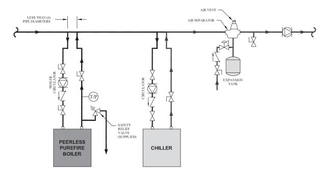
Figure 4.10: Boiler in conjunction with a Chilled Water System
