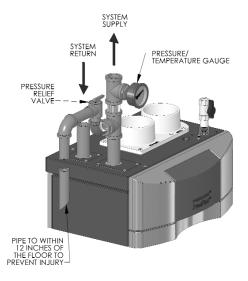
Figure 4.2: Relief Valve Installation – PF-50, PF-80, PF-110 & PF-140
