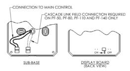
Figure 8.10: Cascade Link Connection & Switch Setting
