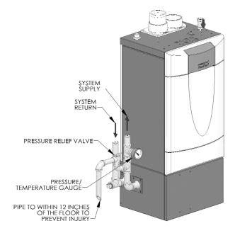
Figure 4.3: Relief Valve Installation - PF-210 & PF-399
