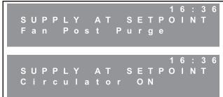
Supply at Setpoint - Fan Post Purge: If the boiler supply temperature exceeds the desired target (either a setpoint or a target calculated by the heating curve) the display will indicate "SUPPLY AT SETPOINT" and show that the boiler has entered the post purge period. After the postpurge, the display will indicate that the boiler circulator (CH PUMP) is operating. The boiler circulator will continue to operate until the demand is satisfied.
