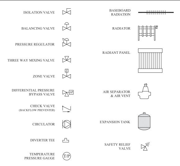
Figure 4.1: Piping Symbol Key
