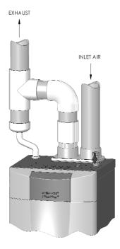
Figure 6.2: Separate Vent Condensate Drain Installation
