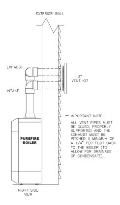
Figure 3.7: Optional Stainless Steel Vent Kit Installation
