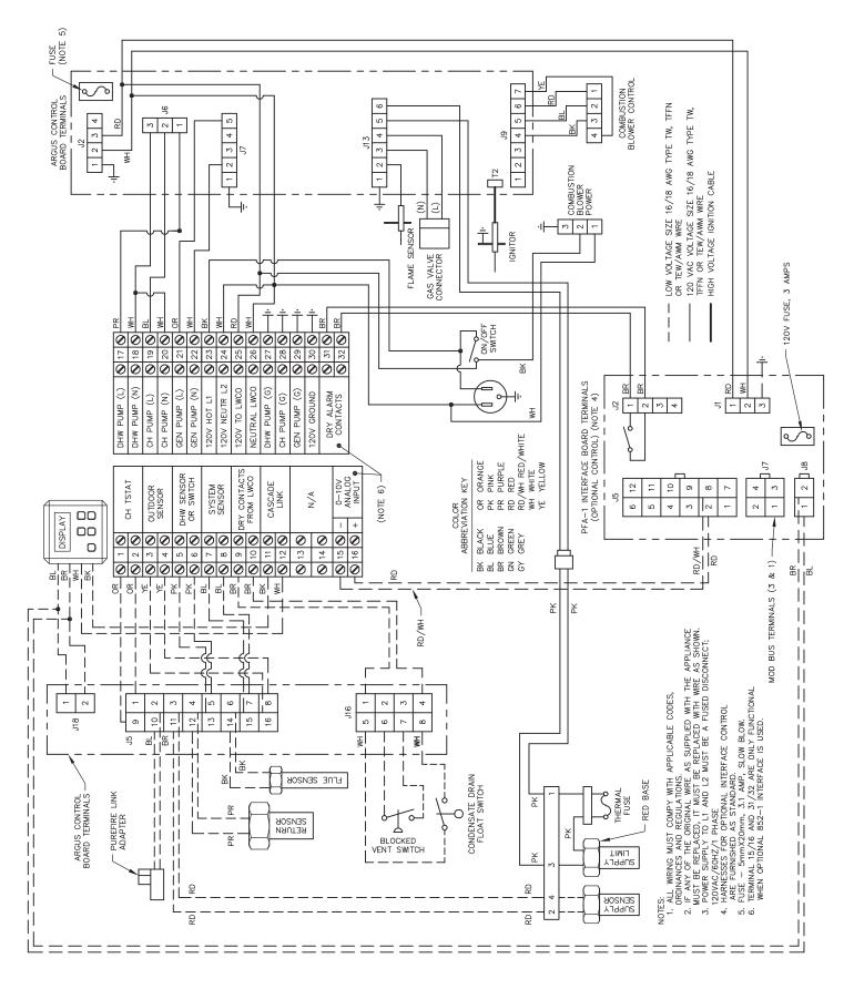
Figure 7.6: Internal Wiring Schematic for PF-210 & PF-399 boilers.
