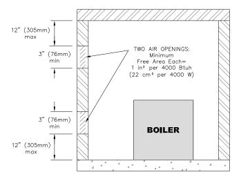
Figure 1.5: Air Openings – All Air Directly from Outdoors
