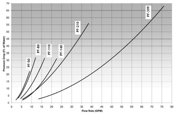
Figure 4.4: PureFire\* Circulator Sizing Graph (General Pump - Primary/Secondary)
