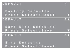
Pressing the "Select" key while viewing this screen allows the installer to reset all values to the factory default settings.
