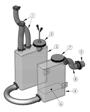
Figure 6.1: Condensate Trap System
