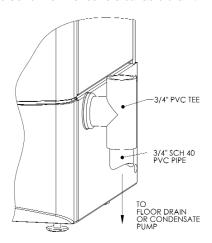
Figure 6.3: Condensate Drain Piping
