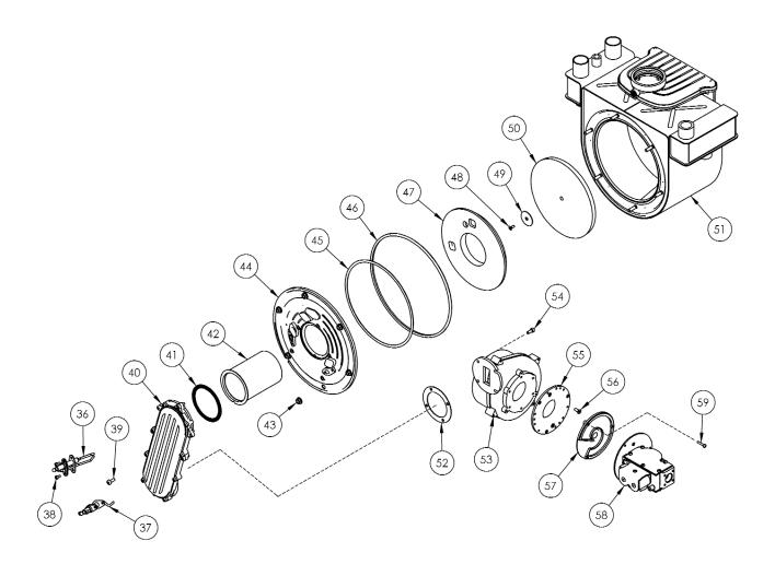
Figure 13.2: Heat Exchanger/Burner Assembly Repair Parts - PF-50, PF-80, PF-110 & PF-140
