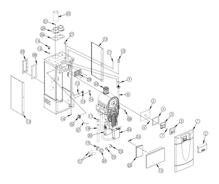
Figure 13.3: General Repair Parts - PF-210 & PF-399
