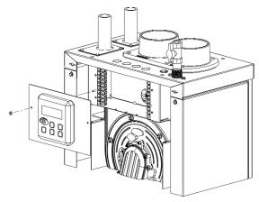
**Figure 7.1: Electrical Terminal Access**
