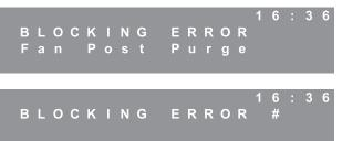
Blocking Error: "Blocking Error" is displayed whenever a condition is reached that prevents the boiler from operating but will not result in a control lockout. Once the condition is corrected, the control will reset automatically. A list of blocking errors is included in Table 10.1.
