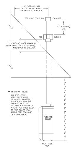
Figure 3.9: Standard Vertical Vent Installation
