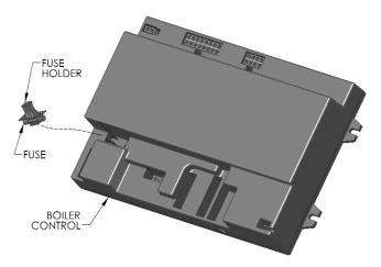
NOTE: BOILER CONTROL HAS A REPLACEABLE FUSE.
