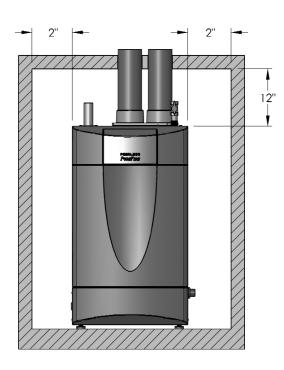
Figure 1.1: Minimum Accessibility Clearances - PF-50, PF-80, PF-110 & PF-140
