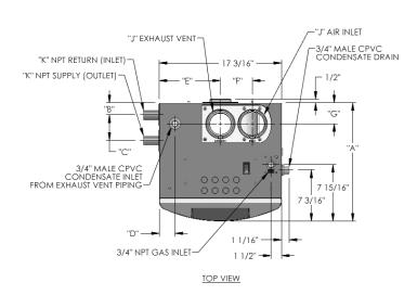
Figure 12.2: Dimensional Drawing - PF-210 & PF-399
