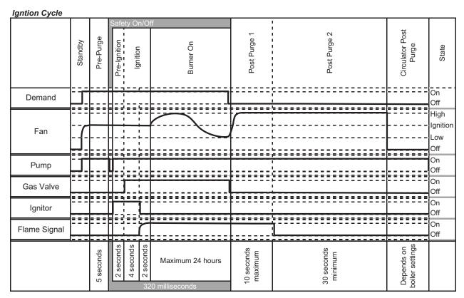
Figure 8.1: Ignition Cycle - Graphical Representation
