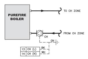
Figure 8.2: Pump Mode = 0, 1, or 2, DHW Mode 0
