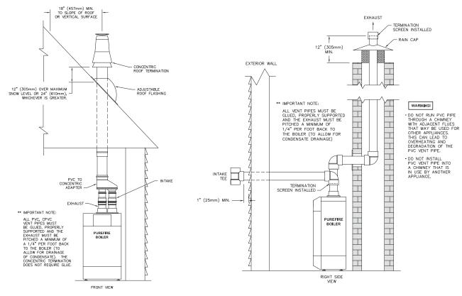
Figure 3.10: Concentric PVC Vertical Vent Installation
