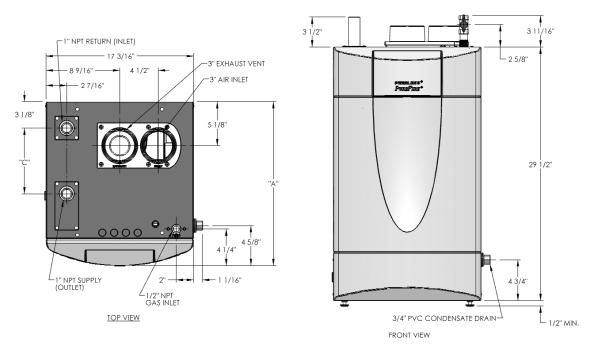
Figure 12.1: Dimensional Drawing - PF-50, PF-80, PF-110 & PF-140
