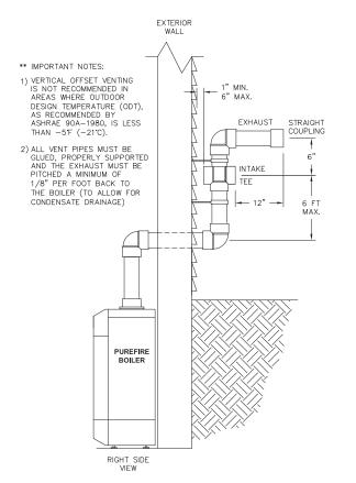
Figure 3.4: Offset Exhaust and Air Inlet Terminations
