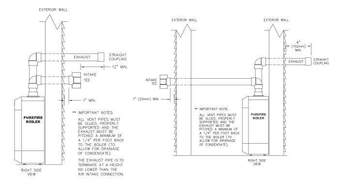
Figure 3.3: Standard Exhaust and Air Inlet Pipe Penetrations
