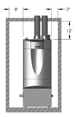
Figure 1.2: Minimum Accessibility Clearances - PF-210 & PF-399
