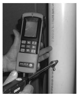
Figure 9.2: Insert Analyzer Test Probe into Test Port
