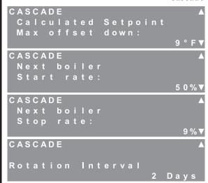
Range: 0 °F to 36 °F Default: 9 °F This is an offset temperature applied to the setpoint of Dependent boilers that the control uses to adjust system response. Higher values increase system response.
