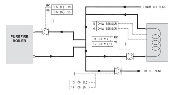
Figure 8.5: Pump Mode = 2, DHW Mode = 1 or 2
