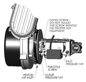
Figure 5.2: Gas Valve/Venturi
