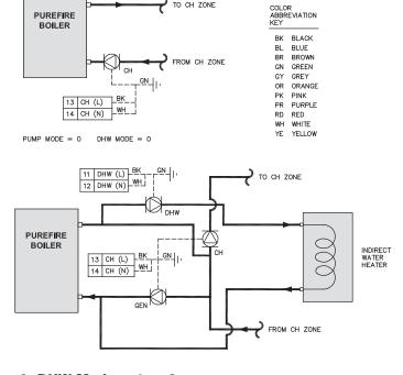
Figure 8.3: Pump Mode = 0, DHW Mode = 1 or 2
