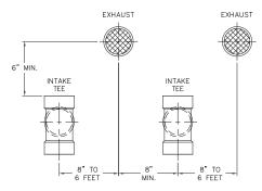
Figure 3.1: Vent Pipe Spacing for Multiple PureFire\* Boilers
