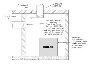
Figure 1.8: Air Openings – All Air from Outdoors through One Opening
