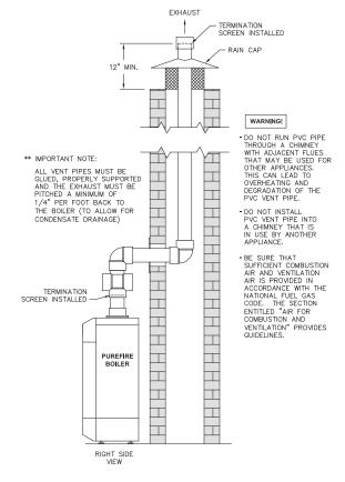
Figure 3.13: Venting with a Chimney Using Inside Air
