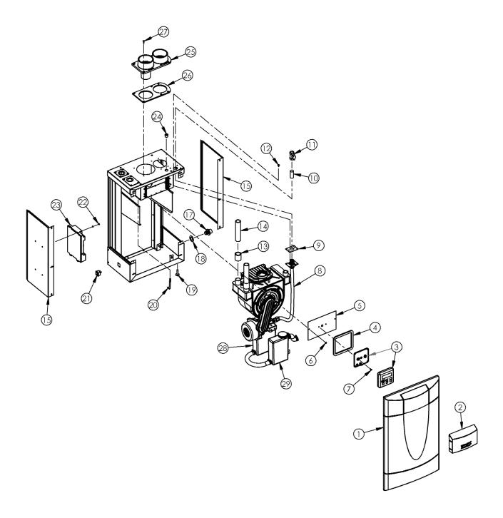
Figure 13.1: General Repair Parts - PF-50, PF-80, PF-110 & PF-140
