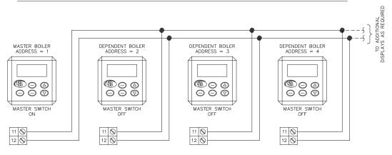
MULTIPLE BOILER CASCADE LINK WIRING: PF-210 AND PF-399
