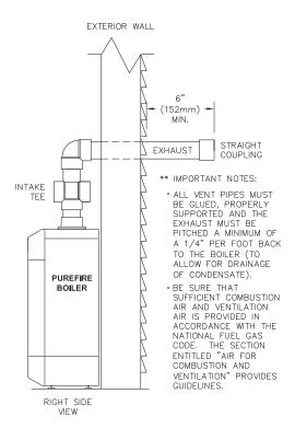
Figure 3.6: Sidewall Exhaust with Indoor Air
