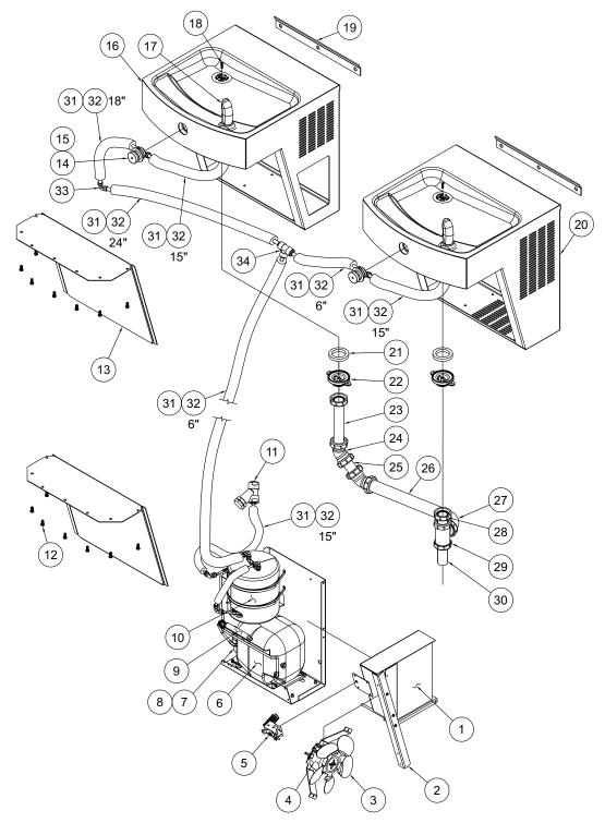
Standard A112.8FGVR series 14 Gage Stainless Steel Enhanced Vandal Resistance Refrigerated Bi-Level shown.
