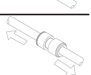
3. Pull on the fitted tubing to ensure it is secure. Tube should not come free from the fitting. Water test the connection assembly prior to leaving the site to ensure there are no leaks.
