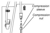
Place the end of the copper tubing into the water valve inlet port. Shape the tubing slightly. Do not kink the tubing so that it feeds straight into the inlet port.
