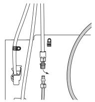
Place the brass nut and sleeve on the end of the copper tube as illustrated. The nut and sleeve are provided in the use and care packet. Do not use an old sleeve.
