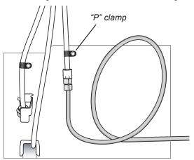
10. Turn on the water supply. Check for leaks and correct if necessary. Continue to observe the water supply connection for two to three hours prior to moving the refrigerator to its permanent location. Monitor the water connection for 24 hours. Correct leaks if necessary.
