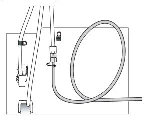
Pull on the tubing to confirm the connection is secure.
