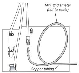
3. Remove the plastic cap from water valve inlet port.
