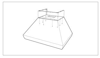
4 Six additional screws are provided to secure the top of the duct cover to an upper cabinet or soffit area, if accessible.
