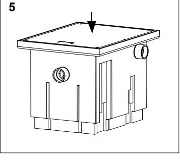
Run sinks to fill unit with water and replace cover. Dispose of grease per local code.
