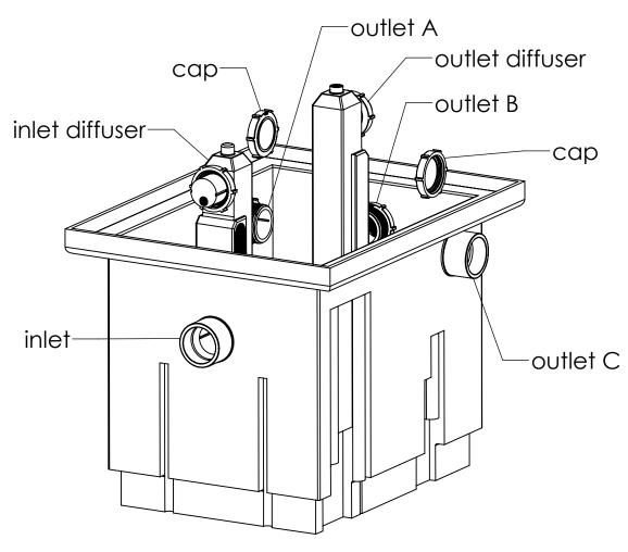
Schier grease interceptors are rated and manufactured with an internal flow control system already in place. They do not require an external flow control fitting.
