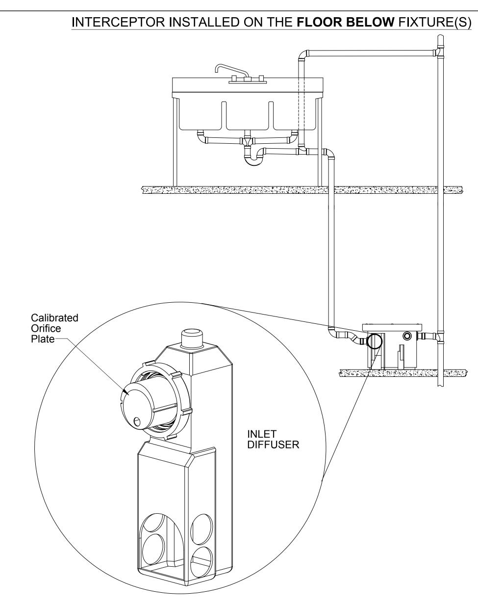
To maintain proper flow rate, keep calibrated orifice plate in place when interceptor is installed on the floor below the fixture(s) it is serving.
