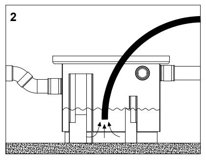
Remove all contents of grease interceptor including grease, sediment and wastewater.
