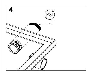
To conduct a pressure test on the pipes, remove diffusers and fasten green caps to the inlet and outlet connections. Do not pressure test unit.
