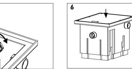
Run sinks to fill unit and replace cover.
