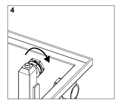
Hand tighten inlet and outlet diffusers back to original positions.
