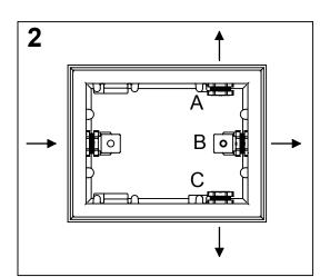
Connect outlet diffuser to the desired outlet (A, B or C). Unit is shipped with outlet diffuser in location B.
