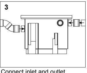
Connect inlet and outlet pipes to unit. Roll down inlet line using (2) 45° elbows immediately preceding the unit to ensure inlet pipe is clear of water.
