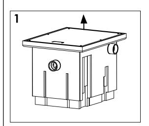
Set unit on level and solid surface near the sink. Remove cover.
