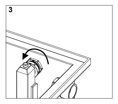
To access the inlet and outlet lines for cleaning, remove the diffusers. Clean diffusers thoroughly before replacing to original position.
