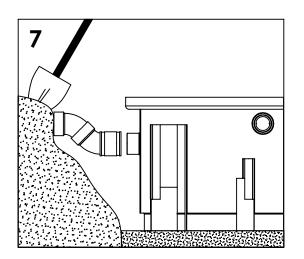
If unit is buried, backfill with sand or pea gravel. Pour concrete and install finished floor. Roll down inlet line using (2) 45° elbows immediately preceding the unit to ensure inlet pipe is clear of water.
