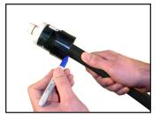
**7** Stab pipe completely into fitting entrance.
