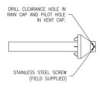
Figure 21. Rain Cap to Small Vent Pipe Assembly
