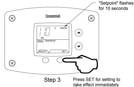
To Change Temperature Format in Display from °F to °C or °C to °F: Step 1: Press "SELECT" button until °F/°C is displayed.
