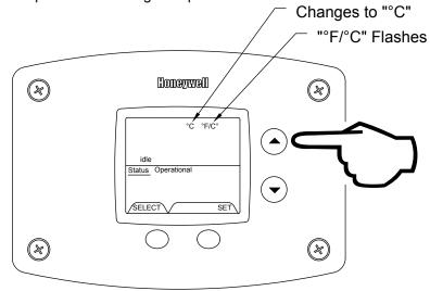
Step 3b: Press "Temperature Down" button to change temperature format to °F.
