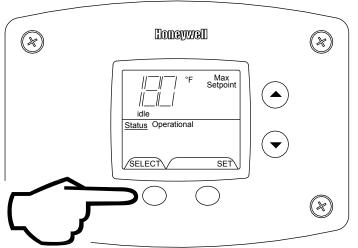
Step 2: Press "Set" button to enter setting mode. "Max Setpoint" will flash to indicate setting mode.
