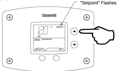
Step 4: To lower the temperature setpoint, press the "Temperature Down" button until the desired temperature is shown on the water heater display.
