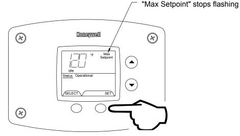
Step 5: 30 Seconds after the last button press, the Water Heater Display will go back to "User Mode". It will read "Max Setpoint" without showing a temperature value if the temperature setpoint is at the maximum setting. The Water Heater Display can be set back to the "User Mode" immediately by pressing both the "Temperature Up" and "Select" buttons together for 3 seconds.
