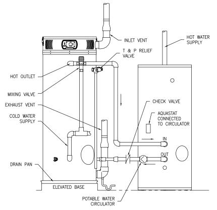
Figure 5. Typical Front Inlet Connect with Storage Heater
