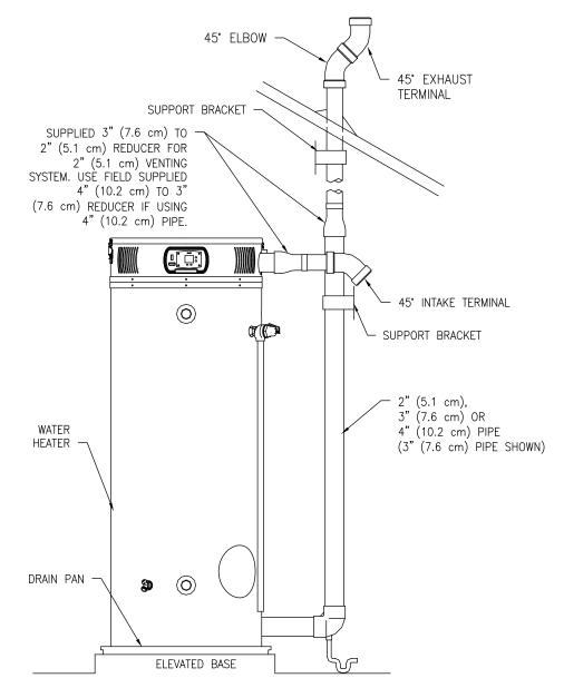
Figure 17. Typical Vertical Power Vent System Installation
