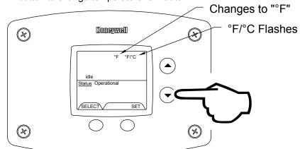
Step 4: Press "SET" button to confirm °F or °C format. °F/°C will stop flashing. Setpoint display will appear in the format selected (°F or °C) in 10 seconds.
