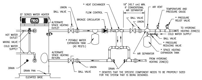
Figure 11. Typical Plumbing Schematic for Zoned Heating
