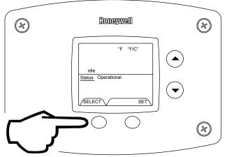
Step 2: Press "Set" button to change temperature format. "F/C" symbol will flash in the water heater display. / "F/C" Flashes
