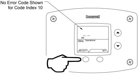
Step 4: Press the "Temperature Down" button to change to the previous code index, code #9.
