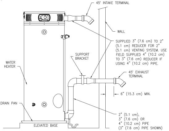
Figure 16. Typical Horizontal Power Vent System
