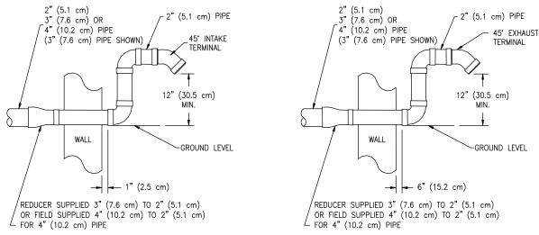
Figure 18. Vent Terminal (Low Ground Clearance)
