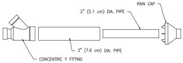
Figure 20. Concentric Vent Kit Part Identification
