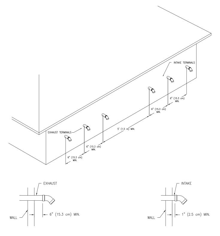
Note: When installing multiple intake/exhaust terminals on the same wall of a building, the nearest intake terminal must be at least 5 feet (1.5 m) from the nearest exhaust terminal.
