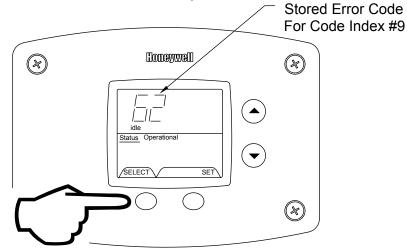
Step 6: Continue pressing the "Temperature Down" button to change to the next error code index and press "Select" to view the error code number, if any, for that index number. Continue on to index #1, the oldest error code index. The water heater display will store up to 10 error codes with the oldest code starting in code index #1 with the most recent code in code index #10.
