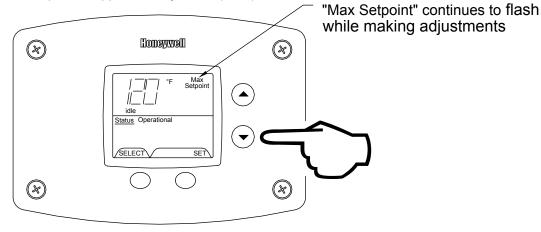
Step 4: Press "Set" button to confirm new "Max Setpoint" value and stop setting mode.
