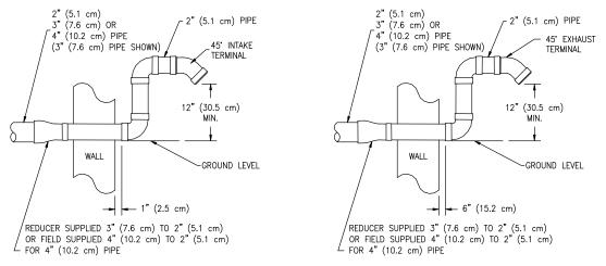
Figure 15. Vent Terminal (Low Ground Clearance)
