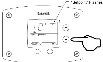
Step 5: When the desired setpoint is reached on the water heater display, press the "Set" button to confirm the new setpoint. "Setpoint" stops flashing in the water heater display.
