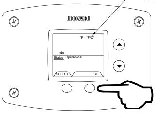
Step 3a: Press "Temperature Up" button to change temperature format to °C.
