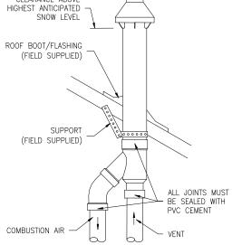
Figure 22. Concentric Vent Roof Top Attachment
