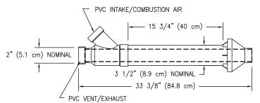
Figure 19. Dimensional Layout of Concentric Vent Kit
