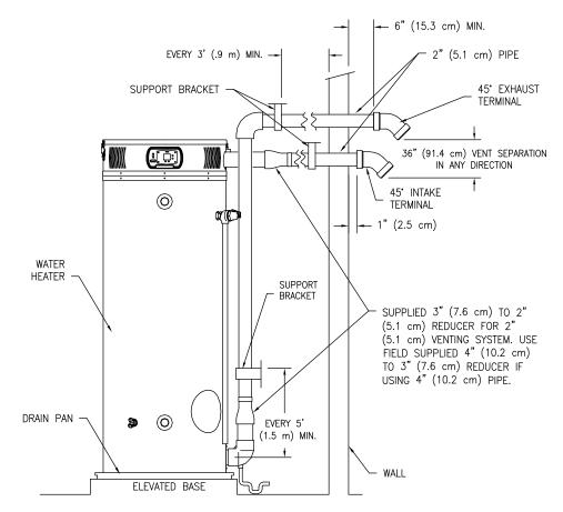
Figure 13. Typical Horizontal Direct Vent System
