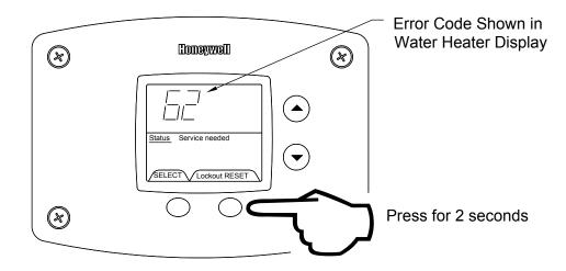
All other error codes will put the water heater into a "Hard Lockout" condition, in which the water heater will not operate and cannot be reset in the "User Mode". To reset a hard lockout, first enter the "Service Mode" described earlier by pressing both the "Temperature Up" and "Select Buttons" at the same time for 3 seconds. Then press the lower right button under "Lockout Reset" in the water heater display and hold for 3 seconds.
