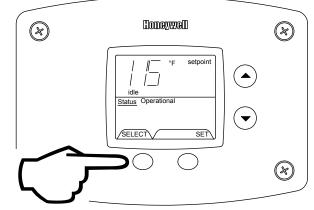
Step 2: Press the "Set" button to enter the setting mode. "Setpoint" will flash in the water heater display.
