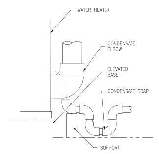
Figure 2. Condensate Elbow With Trap
