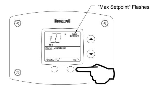
Step 3: Press the "UP" or "DOWN" buttons to change the maximum setpoint value. This will limit the maximum setpoint the user can select. Note: The maximum setpoint is approximately 180°F (82°C).
