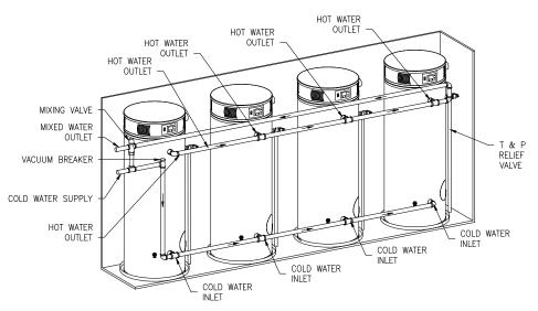
Figure 8. Typical Four Water Heater Connection
