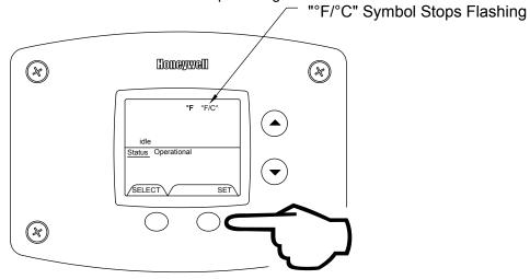
Step 5: Pressing "Select" button will return display to setpoint in format selected (°F or °C) immediately.
