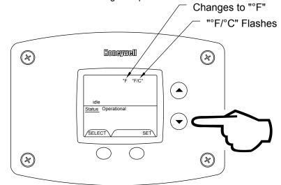
Step 4: Press "Set" button to confirm "F or "C format. "F/"C will stop flashing.
