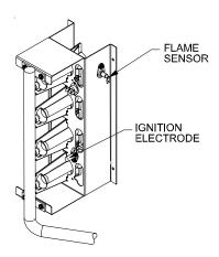
Flame Sensor and Ignition Electrode Location
