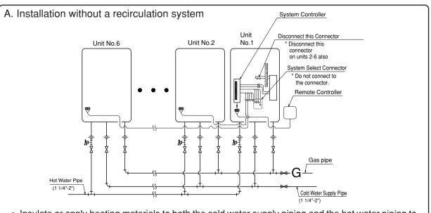
• Insulate or apply heating materials to both the cold water supply piping and the hot water piping to prevent freezing during cold weather and to prevent heat loss through the piping.
