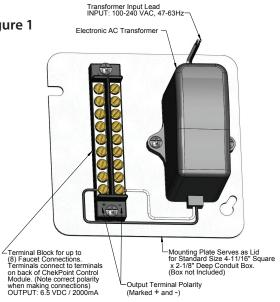
NOTE: Customer is responsible for supplying wiring and installation in accordance with applicable codes
