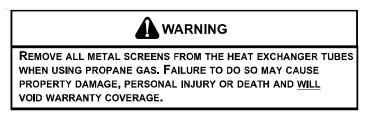
**NOTE:** To prevent premature heat exchanger failure, follow the instructions in the NON-CONDENSING FURNACES AND PACAKGE GAS-ELECTRIC section to remove all metal screen inserts from the entrance of heat exchanger tubes during propane conversions. Not all models will have metal screen inserts.
