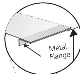
To successfully install the range, the initial level height from floor to underside of cooktop frame should be at least 1/16" taller than cabinet sides as measured in step 2.
