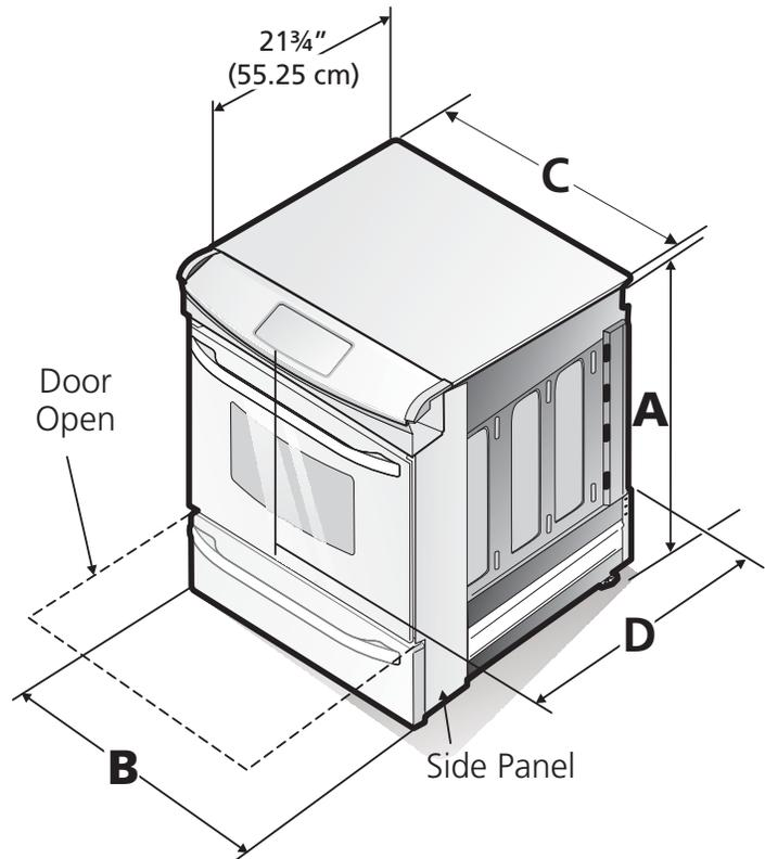
**\* IMPORTANT: To avoid cooktop breakage for cutout width (E dimension) of more than 30 1/16" (76,4 cm), make sure the appliance is centered in the counter opening while pushing into it. Raise leveling legs and the rear adjustable wheels at a higher position than the cabinet height (see page 3), insert the appliance in the counter and then level. Make sure the unit is supported by the leveling legs at the front and the wheels at the back and NOT by the cooktop itself.**
