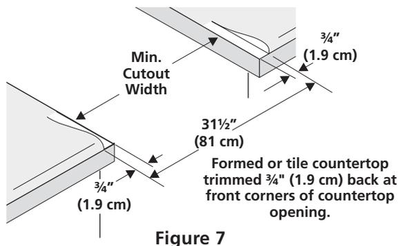
countertop, first side to side, then front to back. If the countertop is not level, the range will not be level. The oven must be level for satisfactory baking results. Cooktop sides of range fit over edges of countertop opening
