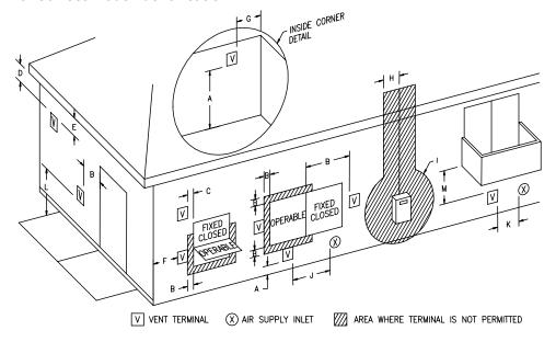
Figure 1 - Vent Terminal Clearances
