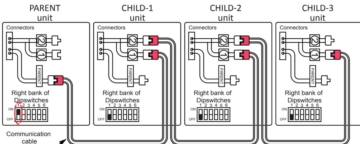
**NOTE:** The dark squares indicate the direction the DIPswitches should be set to.
