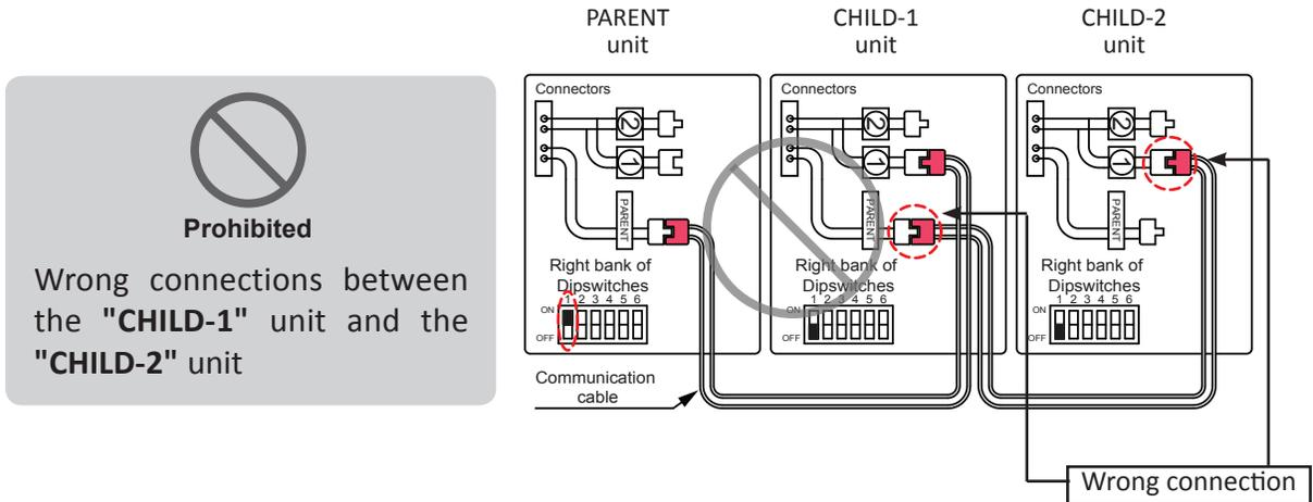
**WARNING** Connecting two "PARENT" connectors together from two separate units **may damage the computer board**. The communication cable has a female end and a male end so it's impossible to have a PARENT-to-PARENT connection with the communication cable. Do not splice or modify connectors.
