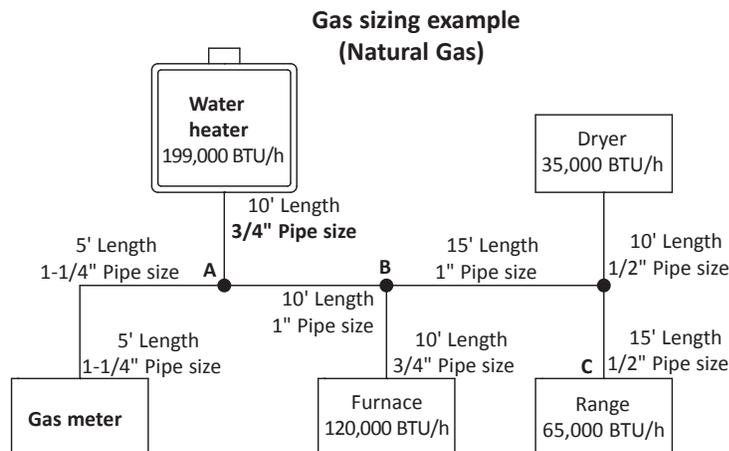
Based on Energy Content of 1,000 BTU/Cubic ft: Divide each appliance's BTU/h requirement by 1,000 BTU/ft<sup>3</sup> to get the appliances ft<sup>3</sup>/h requirement.
