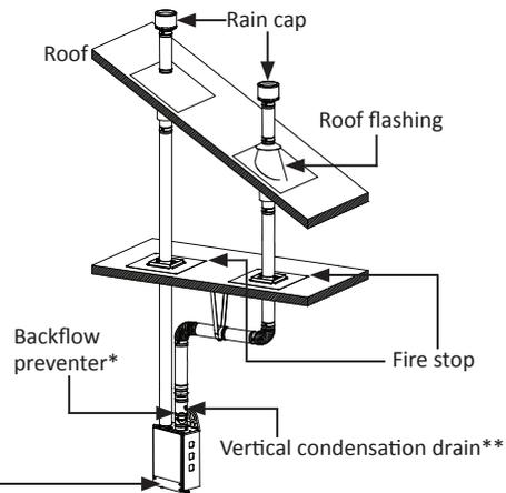
\*Backflow preventer (Recommended for freezing weather conditions: 36 °F (2 °C) and below).
