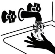
Hot Water Heater temperature over 125 °F (52 °C) can cause severe burns instantly or death from scalding. Children, disabled and the elderly are at the highest risk of being scalded. Feel water temperature before bathing or showering. Temperature limiting valves are available. Ask a professional.
