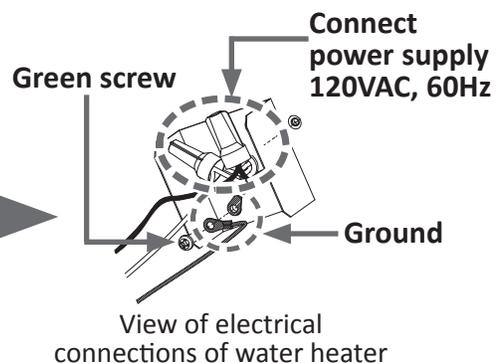
View of electrical connections of water heater
