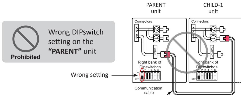
**CASE 2: Wrong connections between the "PARENT" unit and the "CHILD-1" unit**
