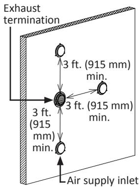
For direct-vent sidewall terminations that use two separate penetrations for the intake and exhaust, distance the intake and exhaust terminations at least 3 ft. (915 mm) away from each other, no matter the orientation.
