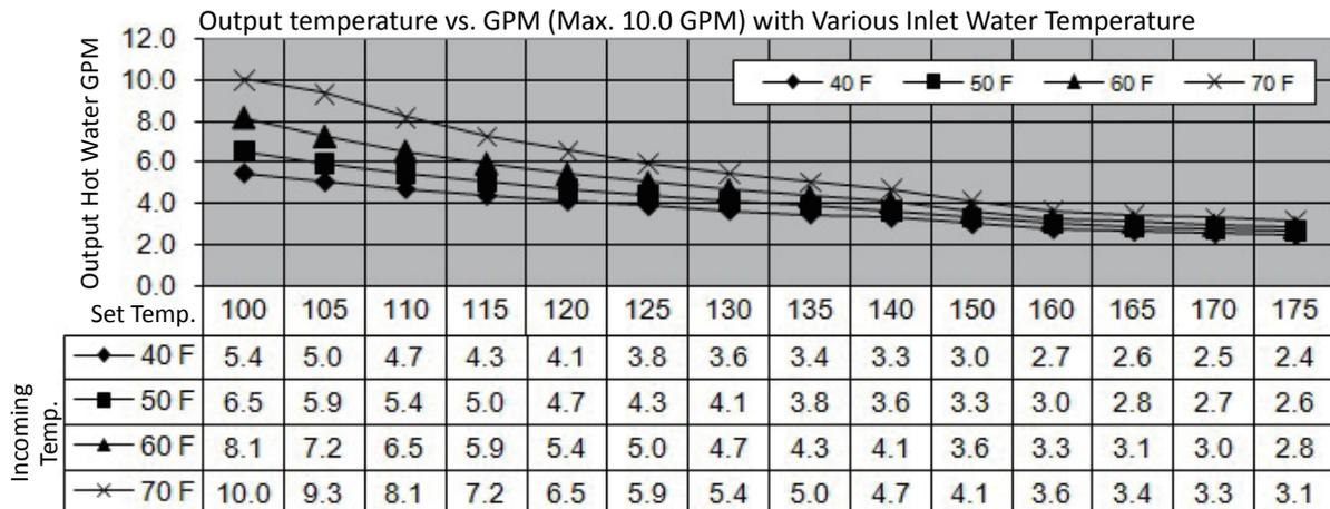
\*When the set temperature is 131 °F or higher, maximum flow rate is limited to 8.0 GPM.
