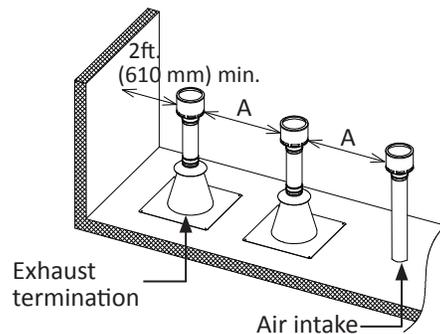
For multiple-unit rooftop terminations (whether for standard or direct-vent installations) space all exhaust and intake terminations in accordance with local codes. An exhaust termination must be spaced from a wall or surface in accordance with local codes as well. In the absence of such a code, an exhaust termination must be a horizontal distance of at least 2 ft. (610 mm) away from a wall or surface.
