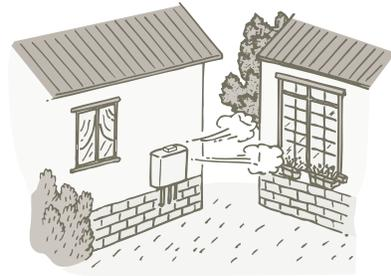
Do not install this water heater under an overhang less than 3 ft. from its top or eaves. The area under an overhang must be open to three sides (Outdoor models only).
